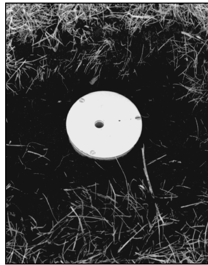
Figure 3.5 Fill In and Pack the Material around the Standard Transducer.
