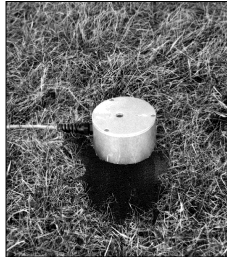
Figure 3.3 Final Installation with Ground Spikes Pushed Fully into the Ground.
